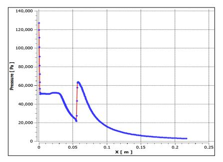
Fig. 6: Pressure variation along the centerline 20-Degree Afterbody with wedge
