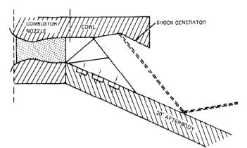
Fig. 1: Sketch Showing Nozzle Separators and cowl
