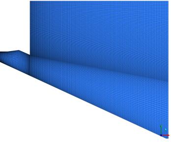
Fig. 3: Quadrilateral Grid for 20-Degree Afterbody
